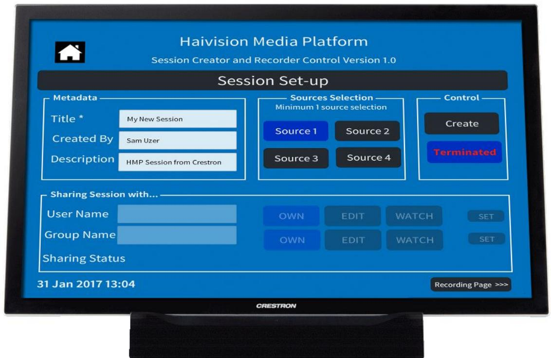
*HMP Driver interface on a Crestron TSD-2020 Touch Screen Control Display*
